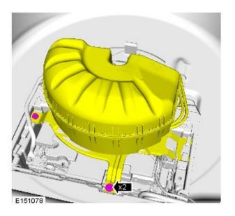
**12.** Connect the battery ground cable and install the spare wheel/tire assembly (see Topix Workshop Manual, Section 414-01).
