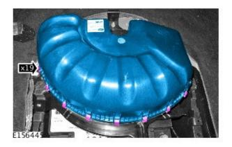
4. NOTE: Do not completely remove the suspension air supply unit from the vehicle; the modification is carried out in the vehicle.
