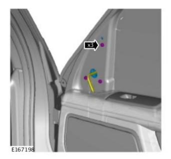
**7.** Install the washers to the door mirror lower retaining bolts only.
