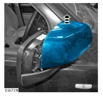
**2.** Check for wear mark damage on the door mirror.
