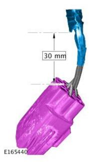
5. NOTE: Make sure the protective sleeve is a minimum of 30mm from the electrical connector.
