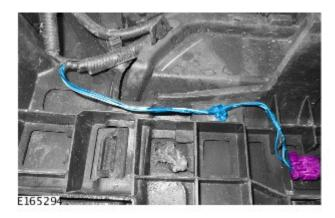
3. NOTE: There must be a minimum of 30mm between the connector and the end of the bumper harness protective sleeve.
