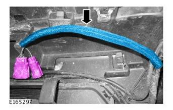
8. NOTE: There must be a minimum of 30mm between the electrical connector and the protective sleeve.
