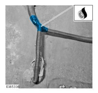
**7.** Wrap the main connector wiring harness in the 4.5mm protective sleeve.
