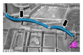
**4.** There must be a minimum of 30mm between the electrical connector and the protective sleeve.
