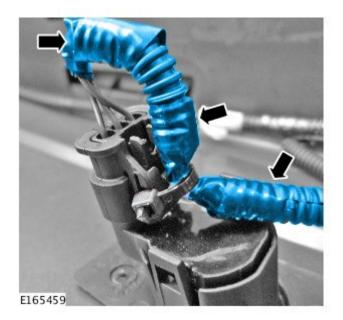
**9.** Secure the rear Parking Aid system sensor wiring harness into the wiring harness channel.
