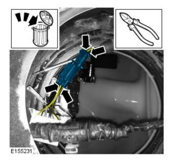
15. CAUTION: After crimping the connection, perform a gentle pull test to make sure that a sufficiently strong connection has been created. If required, remove and replace the splice.
