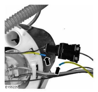
6. CAUTION: After crimping the connection, perform a gentle pull test to make sure that a sufficiently strong connection has been created. If required, remove and replace the splice.
