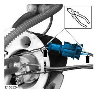
**5.** Using a suitable tool, remove 5mm of insulation from the end of each wire.
