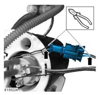
**10.** Using a suitable tool, remove 5mm of insulation from the end of each wire.
