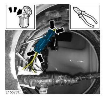
20. CAUTION: After crimping the connection, perform a gentle pull test to make sure that a sufficiently strong connection has been created. If required, remove and replace the splice.
