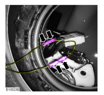
**22.** Measure the resistance values of the fuel gauge sending units.
