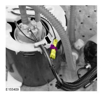
15. CAUTION: Make sure the wiring is cut as close to the connector as possible.
