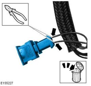
16. Using a suitable tool, remove 5mm of insulation from the end of each wire.
