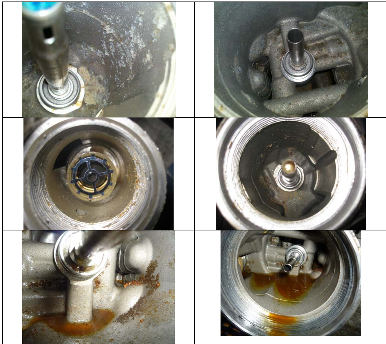
Figure 2 – Examples of Fuel Filter Modules Contaminated with DEF
