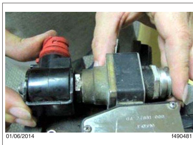
Fig. 2, Separating the Solenoid Valve
