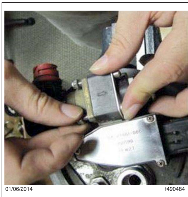
Fig. 5, Assembling the Solenoid Valve
