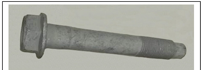
New Bolt: 55080-9FM0A Silver/grey Appearance Torque Value 102.5 N•m ( 75.6 Ft-lbs )
