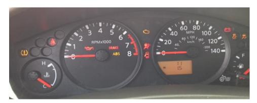
The correct combination meter assembly for Desert Runner models is PN24820-9BF1C. The **correct combination meter** has white faced gauges, satin chrome bezels, and multifunction trip computer functions: Distance to Empty (DTE), Average Vehicle Speed (AVS), Average Fuel Economy (AFE), Elapsed Time (Running Time). The replacement combination meter received from model electronics is shown below.
