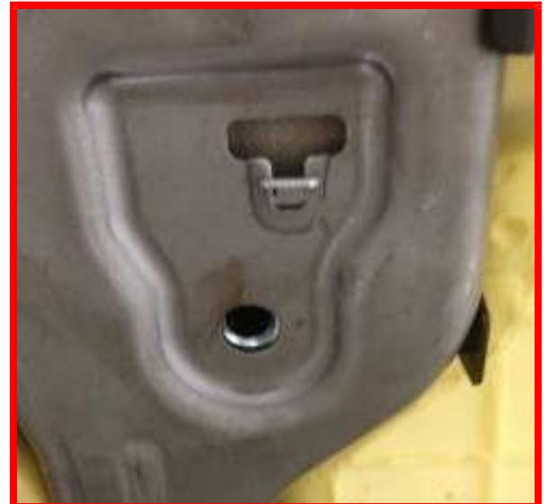
Missing Retractor Bolt
