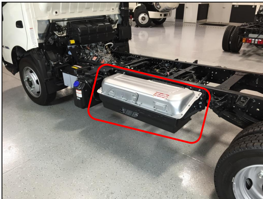
High Voltage Battery Pack Located on Driver's Side Frame Rail
