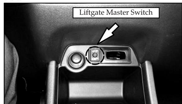
When operating the liftgate using the internal dash mounted switch (left side of the steering column), the liftgate will not open unless ALL doors are unlocked. If only the driver’s door is unlocked, a warning is heard when the switch is pressed and the gate does not open. This does not affect the tailgate mounted switch.
