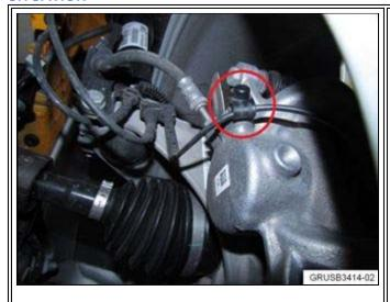
During brake service, the brake pad wear sensor cable may be incorrectly routed and also fastened to the front brake caliper's bleed valve dust cap. Incorrect routing of the brake sensor cable may cause damage to the cable or brake sensor, resulting in a brake warning message being displayed.
