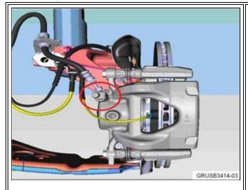
During maintenance brake service, route the brake pad wear sensor cable correctly (as indicated on the illustration).
