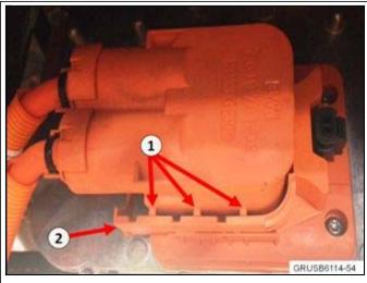
Inspect all HV connectors on the KLE for proper fit. It is possible that one of the HV connectors on the KLE is not seated fully, and in some cases, might not be connected at all.
