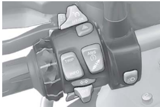
Illustration: Multifunction switch with one-button operation of the turn indicators
