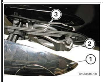
7. Position the exterior door handle slightly outward (1). Feed in the retaining plate (2). Ensure the gasket (3) is seated correctly.
