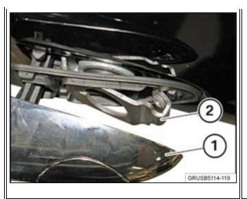
3. Partially pull out the exterior door handle (1). Feed out the retaining plate (2).
