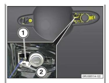
handle and insert properly into the lock actuator (1). Remove the string (2).
