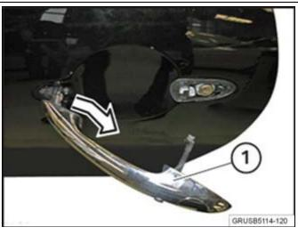
4. Pull the exterior door handle further (1) towards the rear. Feed out the handle from the door. If necessary, unlock the associated plug connections and disconnect; then remove the exterior door handle.
