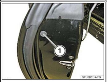
8. Install the retaining bolt and cover plug (1).
