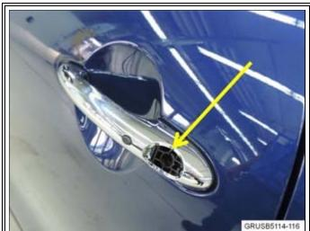
1. The driver's side exterior door handle cover cap is loose or missing.
