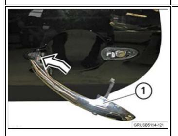
5. To install the driver's exterior door handle, first connect the plug connections; then feed the exterior door handle into the front opening.
