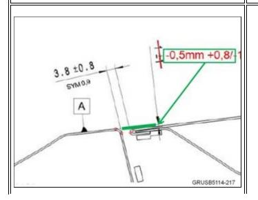
2. In the illustration, the letter A is the rear quarter panel and the other panel is the luggage compartment lid. Adjust the lid locking latch to lower the lid 0.5mm below the quarter panel (A).
