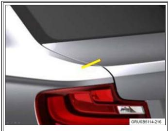
1. Adjust the luggage compartment lid locking latch lower to allow activation of the micro switch.
