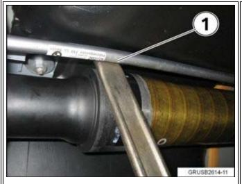
Cold bend the cable tube at point (1).
