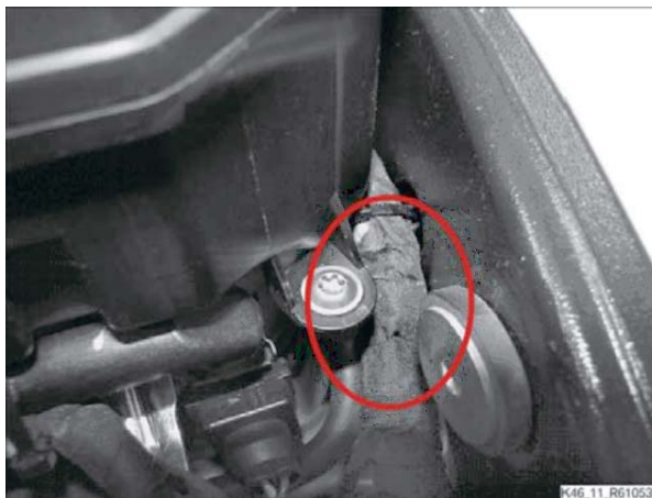
Chafing point on main wiring harness (right side of vehicle)
