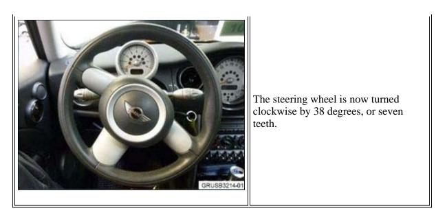
3. Remove the airbag and the steering wheel per Repair Instruction 3233000 (REP-RAR5032-3233000, Removing and installing/replacing steering wheel). Turn the coil spring 38 degrees counterclockwise and bring it into the straight-ahead position. To do this, refer to Repair Instruction 6131006 (REP-RAR5061-6131006, Remove and refit bracket for steering column switch).
