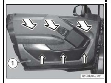
5. Pull the door trim panel (1) away from the door slightly, beginning at the top area. Release the plug connections and cable clips. Remove the door trim panel (1) in an upward direction.
