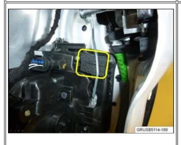
7. Prepare two pieces of the self-adhesive dampening strips (approx. 3 x 8 cm) and apply to the door lock to the area shown.
