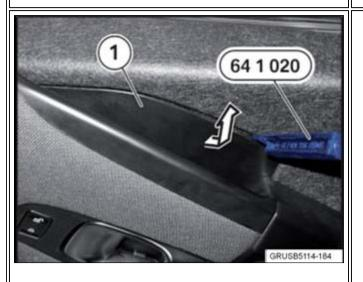
2. Lever out the cover (1) in the direction of the arrow using special tool 64 1 020 and remove.
