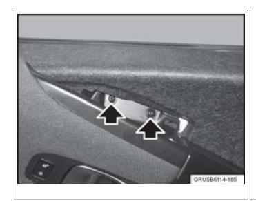
3. Remove the two screws shown.
