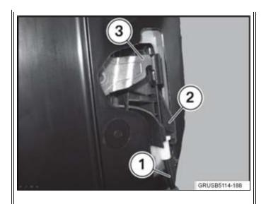
Perform a function check for the inside door handle with the door open and rotary striker lock closed.
