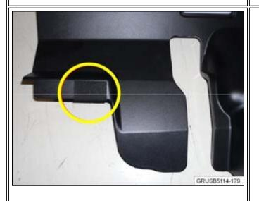
2. Prepare a piece of felt tape (70 mm x 40 mm) and apply the felt so that half of the felt can be wrapped around to the rear area. Shown is the proper location for the front area of the felt.
