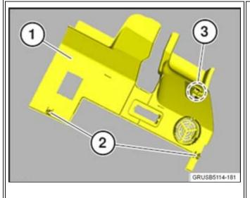
4. Installation note: The clamps (2) and the guide (3) on the trim panel (1) must not be damaged. Insert the guide (3) correctly into the corresponding holder on the vehicle.
