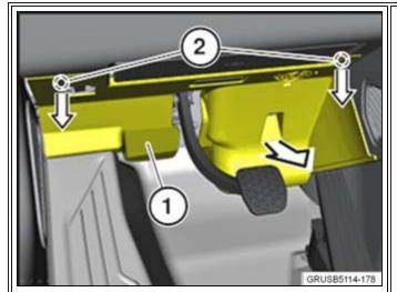
1. Unclip the trim panel (1) from the clamps (2). Lower the trim panel (1) slightly and disconnect the plug connections from behind. Pull out the trim panel (1) towards the rear.
