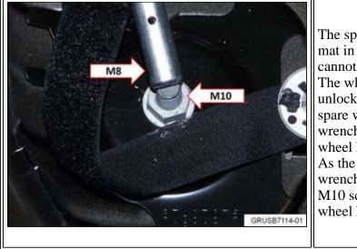
The spare wheel holder under the floor mat in the luggage compartment cannot be removed. The wheel bolt wrench is required to unlock and remove the bolts from the spare wheel. To do this, the wheel bolt wrench is screwed onto the spare wheel holder (thread diameter M10). As the thread size of the wheel bolt wrench is M8, it cannot be used for the M10 screw connection of the spare wheel holder.
