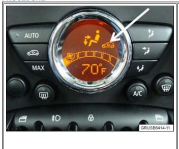
1. The recirculation display is shown when the recirculation button is pushed. It will automatically switch recirculation off after a few minutes, depending on interior and exterior temperatures, to allow fresh air to enter the cabin. This feature was added to reduce the amount of condensation and fogging on the inside of the windows.
