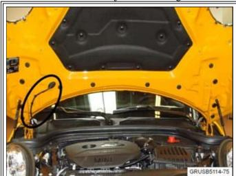
1. Open the bonnet. Locate the washer hose to be modified near the passenger's side gas strut, attached to the bonnet. See the area circled in black.
