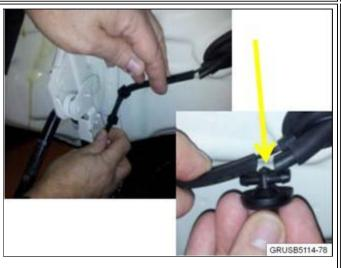
4. Pull the washer hose back far enough to install the pulsation dampener. Do not damage the attached wiring.
