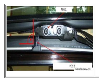
6. With the glass sunroof panel in the lifted position, check the position of the glass sunroof guide (position 2). This should be positioned as shown. Correct as needed.
