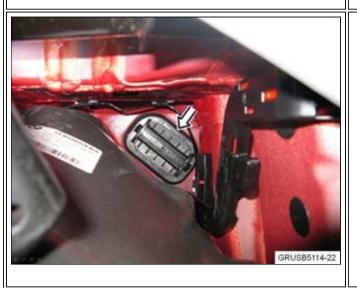
5. To remove the drain plug, follow the arrow direction and pull out downwards. Discard the drain plug.
