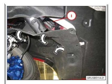
E-box drain plug (1) from underneath the vehicle.
