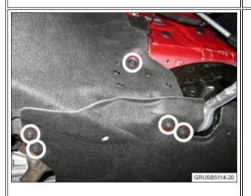
3. Remove the five fasteners as shown.
