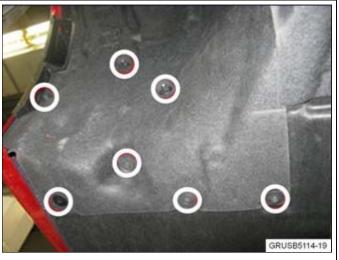
2. Remove the seven fasteners as shown.
