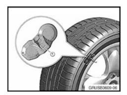
New style wheel electronics The wheel electronics consist of a plastic housing with integrated circuitry. The following items are contained within the wheel electronics: Pressure sensor Temperature sensor Acceleration sensor Transmitter/receiver unit Self-diagnosis controller Battery
