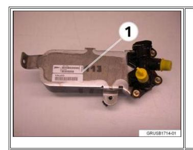
• Access the cooler and visually check the parts label on the coolant side of the cooler (1).
