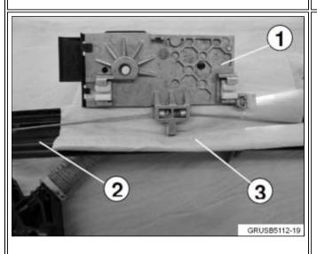
4. Use a protective rag (3), and lay the slider (1) on the rail (2).
