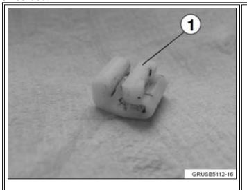
1. Locate the nylon guide clips (1) on the window regulator, and replace the clips using the following steps.
