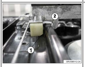
9. Check that the bump stop (1) is contacting the rail (2). Clean the rail and apply a small amount of grease to both rails. Repeat the same procedure for the opposite slider.
