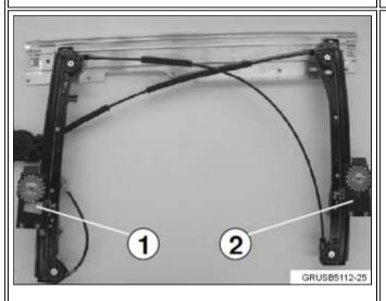
10. After all four guide clips are installed into the sliders of both rails, clean and lightly grease the rails. Install the regulator, and quality check the repair by cycling the window up and down for noise-free and proper operation.
