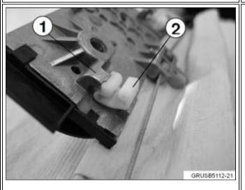
6. Insert a new clip (2) into the top recess of the slider (1), and push down firmly until it snaps in securely. Use the same guide replacement procedure for the other end of the slider.
