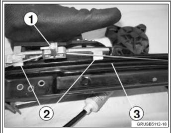
3. Pull the slider (1) outwards, and unclip the nylon guides (2) from the rail (3).
