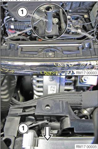
Unlock the fan shroud on the right side (1) in the direction of the arrow.
