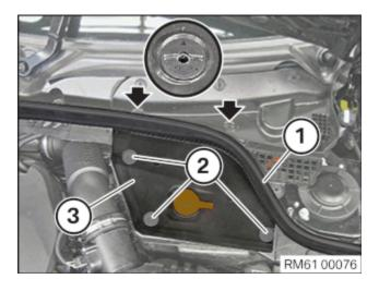
Install the battery cover (3) and tighten the screws (2).
