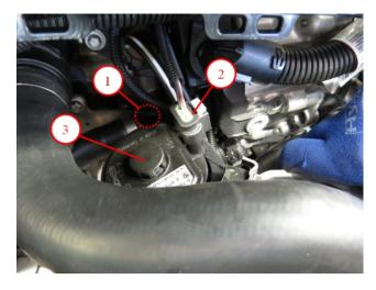
Release and remove the connection (1).
