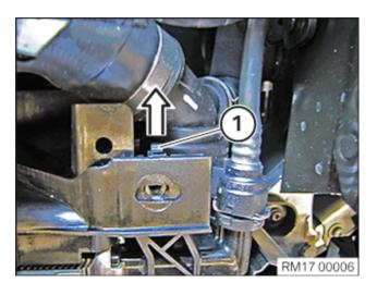
Unlock the left side of the fan shroud (1) in the direction of the arrow.
