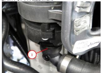
April 14, 2014 Release and remove the hose connection (1).
