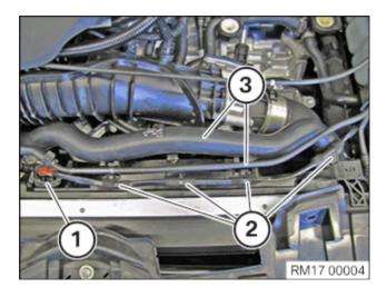
Connect the electrical plug (1) at the fan shroud plug socket.
