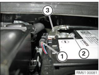
Unlock and disconnect the connector (1).
