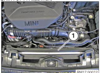
April 14, 2014 Reinstall the gasket/seal (1) on the radiator.
