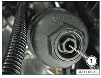
Loosen the oil filter cap drain plug (1) and drain the engine oil from the housing.
