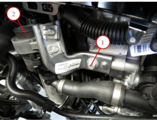
Remove the auxiliary water pump:
