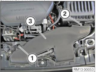
April 14, 2014 Remove the intake duct:
