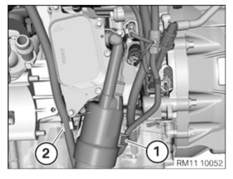
Clip the wiring harness (1) back together.
