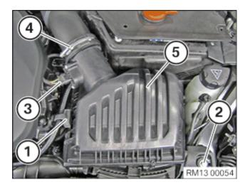
Install the intake silencer and intake duct:
