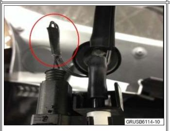
11. This step is only for vehicles equipped with heated washer nozzles. Tape off the extra cable for the heated washer nozzle as shown.
