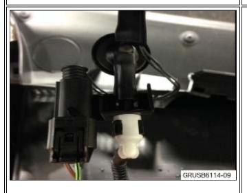
10. Reinstall the washer connection back onto the clip as shown.
