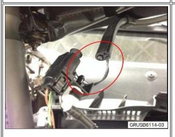
4. Disconnect the washer jet hose from the hose connection elbow and clip, as shown.
