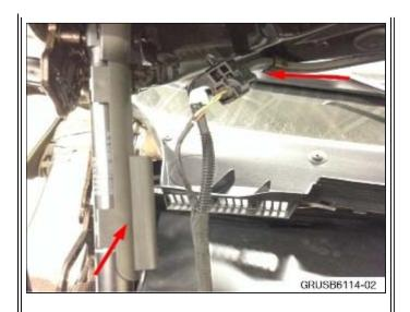
harness from the gas strut, and release the clip from the hood.
