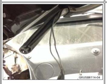
5. Only perform this step if heated washer nozzles are equipped. Remove the wiring harness from the hose as shown.
