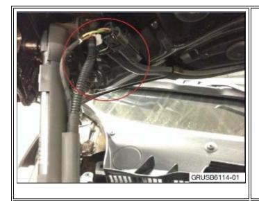
2. The area to be repaired is highlighted near the hood gas strut on the passenger's side of the vehicle.
