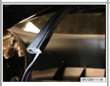
7. This step is only for vehicles equipped with heated washer nozzles. Reinstall the harness back into the groove in the hose, as shown.
