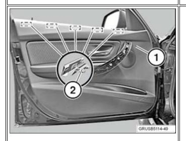
4. Pull the door trim panel (1) off the clamps (2) in an inward direction.
