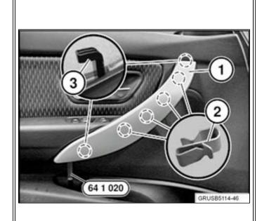
1. Working from the bottom, unclip the cover (1) from the clamps (2) and the latch mechanisms with special tool 64 1 020.
