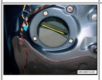
10. With a clean rag, reach through the speaker opening and clean the outside area of the lower part of the window. Remove the protective tape from the selfadhesive seal and apply it to the outside of the window in the position shown. The seal will direct the water away from the rear of the loudspeaker.
