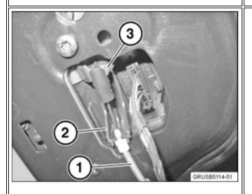
6. Disengage the Bowden cable (1) for the release lever first at the counter support (2), and then at the door lock (3).
