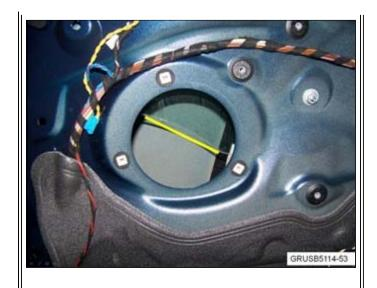
lower edge of the glass can be easily accessed through the speaker opening, as shown.
