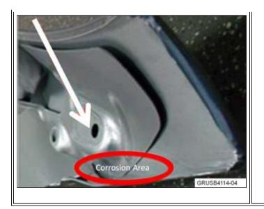
The white arrow shows where the cavity spray tube will protrude after being inserted from the top. The red circle shows the area needing the additional corrosion protection spray.
