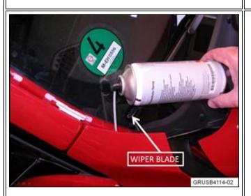
4. Shake the cavity protection spray can for at least 30 seconds.
