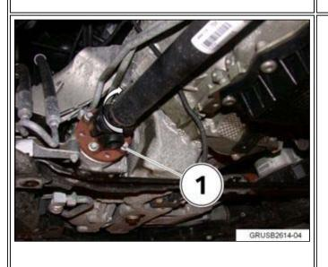
3. Rotate the driveshaft 90° and repeat steps 1 and 2. Rotate the driveshaft another 90° and recheck for play. Rotate a total of four times (the driveshaft has now been rotated 360° total). There should be no play in the U-joints.
