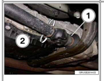
2. Checking the Rear U-joint:
