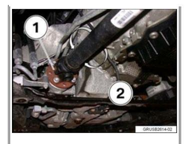
1. Checking the Front U-joint:
