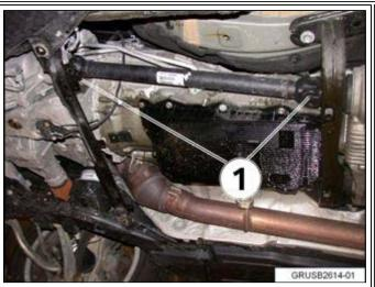
Check the universal joints in the front driveshaft for axial play (1). Note: The E72 will need to have the reinforcement plate removed to check the driveshaft U-joints. Refer to Repair Instruction 31 10 010, "Removing and installing/replacing reinforcement plate."
