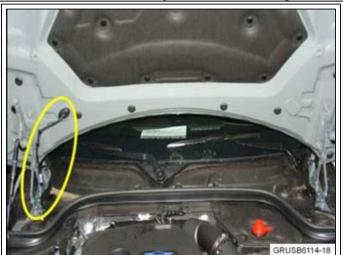
1. Open the bonnet and locate the washer hose to be replaced near the passenger's side gas strut, attached to the bonnet.
