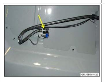
5. Fold the bonnet insulation upward to gain access to the washer hose and electrical connections. Disconnect all connections from both washer jets and all the remaining black plastic securing clips from the bonnet. Work the hose, wiring connectors and grommet from the bonnet and discard.
