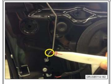
Locate the door lock rod and the area where the felt tape will be applied. Prepare a piece of felt tape 20 mm long by 10 mm wide. Clean the area with a rag. Wrap the felt tape to the area shown. Reinstall the removed door panel in the reverse order of its removal.
