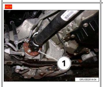
3. Rotate the driveshaft 90° and repeat steps 1 and 2. Rotate the driveshaft another 90° and recheck for play. Rotate a total of four times (the driveshaft has now been rotated 360° total). There should be no excessive play in the U-joints.
