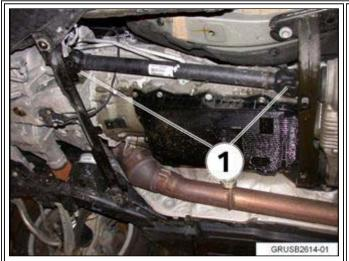
Check the universal joints in the front driveshaft for radial play (1). Note: The E72 will need to have the reinforcement plate removed to check the driveshaft U-joints. Refer to Repair Instruction 31 10 010, "Removing and installing/replacing reinforcement plate."
