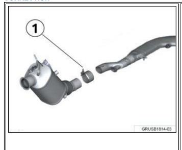
The band clamp (1) is a one-time use only part. It must be replaced after any work performed that requires removal of the exhaust. The clamp will not hold its tightening torque when reused.
