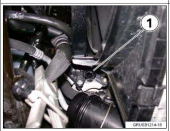
After clamping, remove the outflow hose from the heat exchanger (1).
