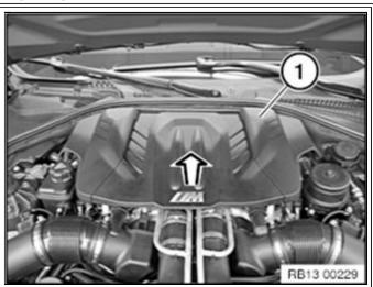
Unclip the engine cover (1) toward the top and remove.
