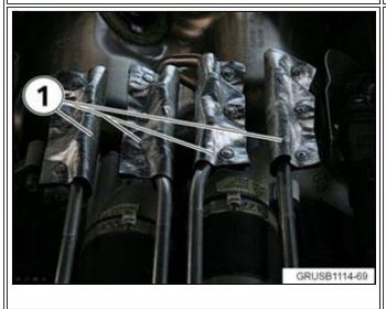
Install insulator sleeves (1) on all four coolant lines as shown. Insulator sleeves are to be installed on the original coolant lines (no leaks found) or after replacing the coolant lines (leaks were found).
