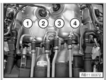
delivery line and coolant return line if there any leaks are found. Follow Repair Instruction RA 11 53 ... "Removing and installing/replacing coolant flow pipe and coolant return pipe for exhaust turbocharger (S63T 0) for coolant line replacement."
