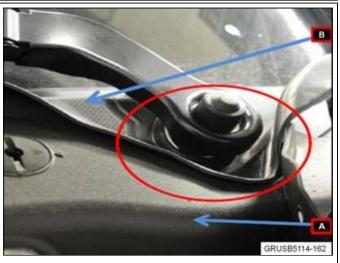
3. The close-up picture shows the correct cowl trim overlap. Reposition as needed.
