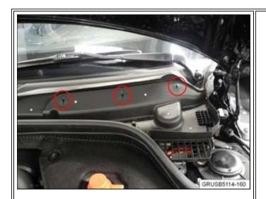
1. Check the three locking toggle fasteners on the driver's side trim cowl for correct installation.
