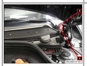
4. Check that the securing lug is fully hooked in. The hook on the small left cowl panel trim (B) must be pushed under the large cowl trim (A).
