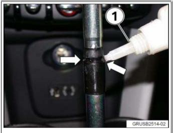
Apply one drop of adhesive (1) to each side of the groove.
