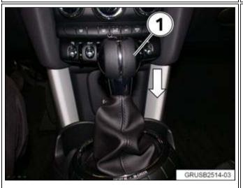
Reinsert the shifter knob (1), making sure the shift gate schematic is in the correct position. Use a padded glove to knock the shifter knob back into position.
