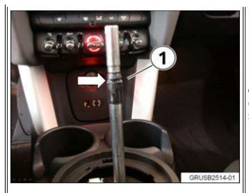
Only apply the adhesive to the groove (1) of the plastic sleeve on the shifter rod. Do not over-apply the adhesive.
