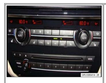
1. The customer A/C settings are typically below 63 deg F with a low fan setting of one or two LEDs.
