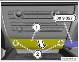
2. Remove the cover (1) using special tool 00 9 327 at the latch mechanisms (2), and remove the cover in the direction of the arrow.
