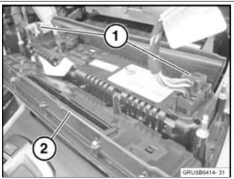
4. Rotate the control panel downward to expose the plug connection (1) on the passenger's side.
