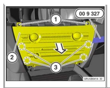
3. Remove the screws (1), radio and IHKA controls (2) using special tool 00 9 327 at the latch mechanisms (3).
