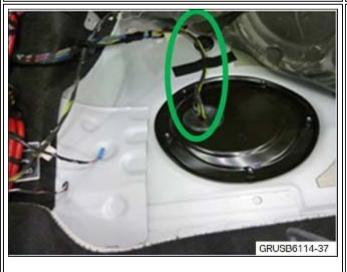
If the harness is routed and secured (taped) as shown, no further action is required.
