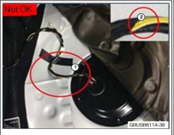
If the harness is routed as shown (1), inspect the harness for any damage (2) and repair as needed.
