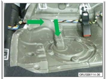
Lift up the insulation under the rear seat. The arrows indicate where the harness runs under the insulation.
