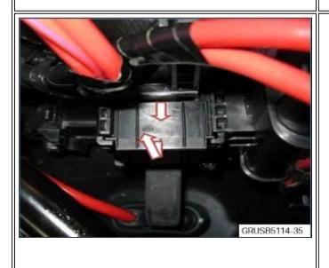
• Remove the cover on the battery positive terminal in the direction of the arrow, and replace it.
