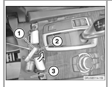
3. Insert the metal key into the lock (1) and turn in the direction of the arrow to the left. Carefully work the lock cylinder (2) upwards with a suitable prying tool and remove the lock from the center armrest (3).
