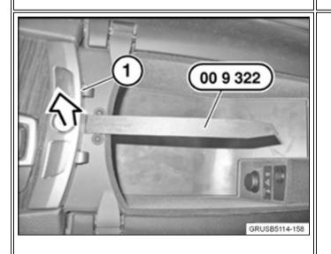
2. Open both center console doors. Carefully lever out the center armrest lock trim (1) from the center console with special tool 00 9 322 and remove.
