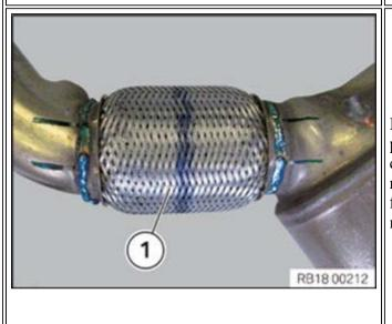
ISTA/D also has an associated repair procedure for replacing this flexible coupling (1). The repair involves removing the DPF; cutting out the old flexible coupling; and welding in the new part.
