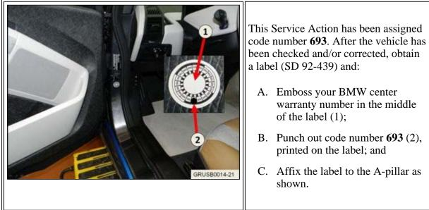
If the vehicle already has a label from a previous Service Action/Recall Campaign, affix the new label next to the old one. Do not affix one label on top of another one because a number from an underlying label could appear in the punched-out hole of the new label.
